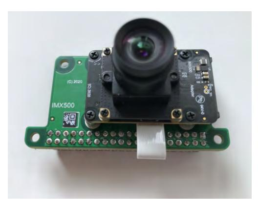
The FR-EK consists of a Raspberry Pi CPU board, the SONY IMX500 Type 2 camera module, and the Xailient FR SDK. The FR solution is capable of fast, high-accuracy FR in both single-face and multi-face modalities under a broad range of real-world conditions.
